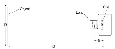
Figure 6. Imaging Field of View
